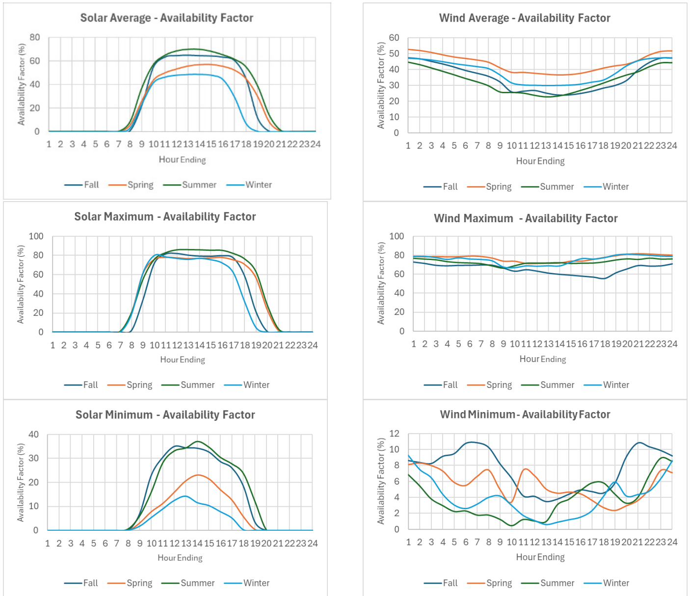
2025 ERCOT Hourly Average, Minimum, and Maximum Availability Factor of Wind and Solar Generation
