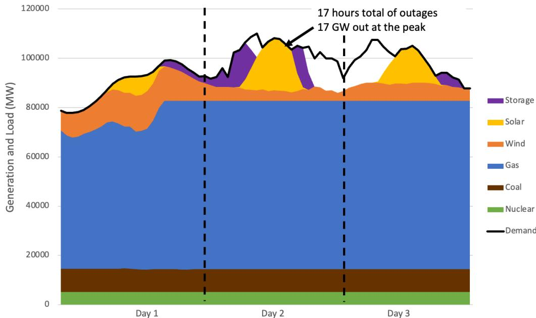
**Note:** Generation forecasts are derived by scaling the generation output in **Figure 2** in Part One of this series to match the installed capacities in **Figure 1** in this paper. The demand forecast is derived by scaling the demand profile in **Figure 2** in Part One of this series to a peak demand of 110 GW.
