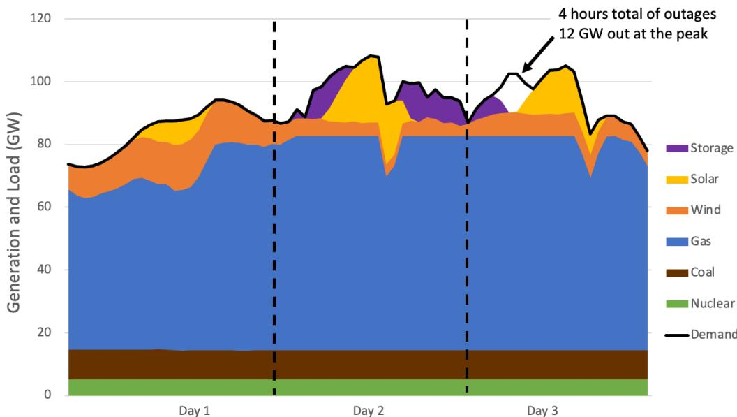
**Note:** This figure is derived by using the same initial data as in **Figure 2** and reducing demand by 5 GW for the entire period.
